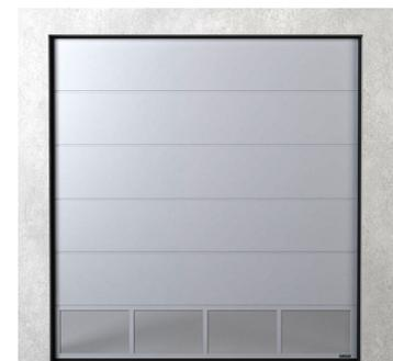
Aluminium panel infilled with a single layer of galvanized expanded steel mesh or double layer of galvanized perforated steel sheet. The panel is painted on both sides in the external door colour.
