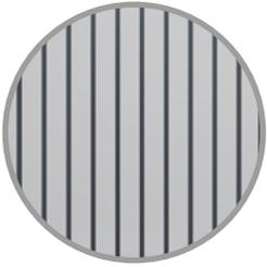
Round tube section infill  $\varnothing$  25mm welded to the structure.
