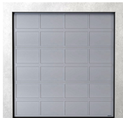
◀ MakroPro ALU 2.0 ELH door with an aluminium panel without a thermal break, with an aluminium sheet-expanded polystyrene-aluminium sheet infill.
